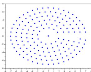
Figure 4: Circular path coordinates created in Scilab and output in format for input to the Mobility.cpp algorithm in ROS.
