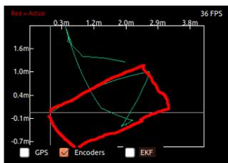
Figure 7 – Kalman Filter versus Actual Route
