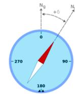
Figure 5 - Example of Magnetic Declination
